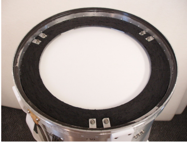
Fig. 5.3.4. 30-cm polyethylene lens, the primary optics for the BICEP telescope. This lens is anti-reflection coated with an expanded polyethylene sheet bonded to the polyethylene surface. More highly curved lenses were coated for the QUAD experiment using the same technique.
