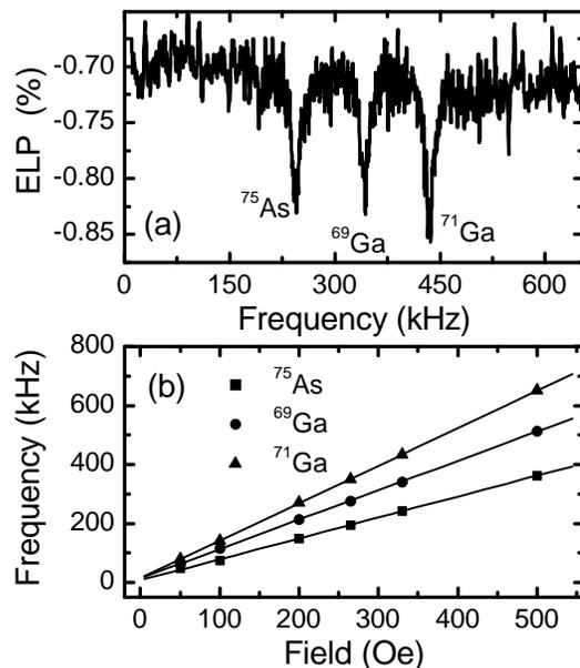
FIG. 3: (a) Frequency-swept NMR depolarization features at  $T = 20$  K,  $H_0 = 330$  Oe, and  $H_1 \approx 0.2$  Oe, corresponding to the three isotopes present in the GaAs QW. (b) Depolarization peak frequency as a function of  $H_0$  at 20 K and  $H_1 \approx 0.2$  Oe. The solid lines are linear fits.
