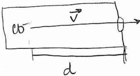
QUESTION: Find the direction and magnitude of the electric field needed to move the CO molecules through the hole at  $8 \times 10^4$  m/s
