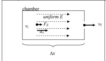
$v_i$ = 0; initial velocity of the  $CO^+$  molecule  $v_f$ =8x10<sup>4</sup>m/s; final velocity of the  $CO^+$  molecule E: uniform electric field in the chamber  $\Delta x$  =0.8m; distance to hole in chamber q=1.602x10<sup>-19</sup>C; charge of a  $CO^+$  molecule m=mass of a  $CO^+$  molecule  $a_x$ =acceleration of the  $CO^+$  molecule in the uniform electric field
