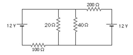
28. *Electric Power:* As part of your summer job as a design engineer at an electronics company, you have been asked to inspect the circuit shown below. The resistors are rated at 0.5 Watts, which means they burn-up if more than 0.5 Watts of power passes through them. Will the  $100\Omega$  resistor in the circuit burn-up?
