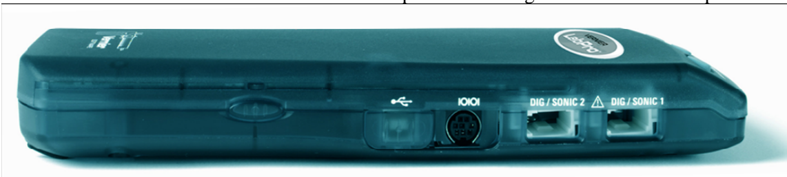
Serial Port and Digital Channels (USB Port is behind the sliding door)
