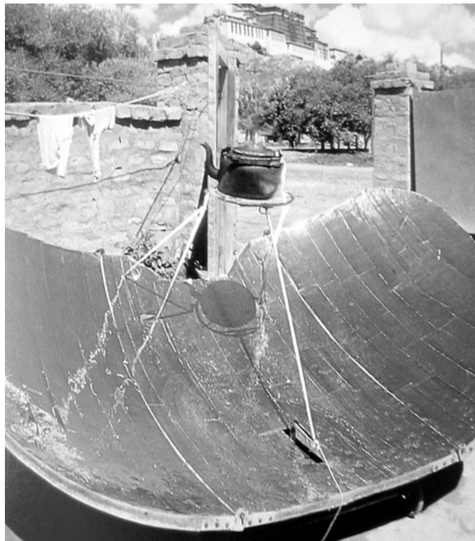
A parabolic mirror uses the sun's rays to boil a kettle of water in Tibet.
