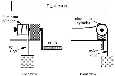
Your device consists of an aluminum cylinder that can be turned with a crank. A rope is wrapped around the cylinder a few times so that, as the crank is turned, the friction between the rope and cylinder is just enough to support a heavy block hanging from one end of the rope. For safety, the other end of the rope is held loosely such that no force is exerted on that end of the rope.
