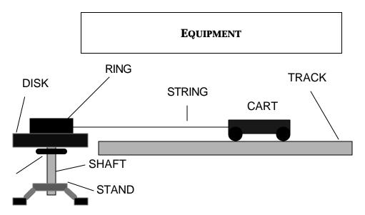
You will have a disk mounted horizontally on a sturdy stand, with a ring coaxially fastened on the disk. Together, the disk and the ring represent the flywheel. The disk and the ring rotate freely about a vertical shaft through their center.
