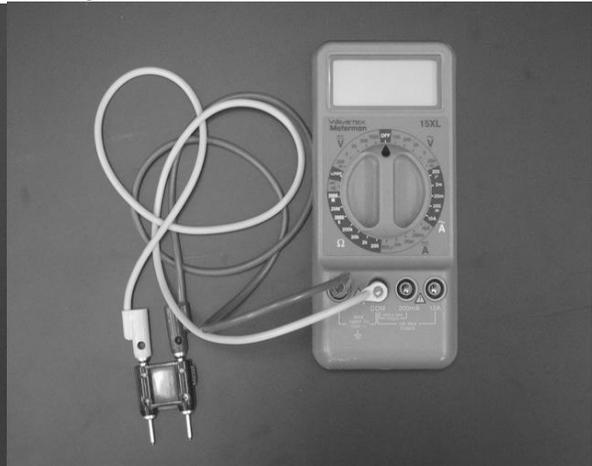
To measure the electric field from the charged electrodes, you will use a probe connected to a digital Multimeter set to measure volts (see Figure 2). For best results, turn the DMM to measure in the two-volt DC range, as indicated in Figure 2.
