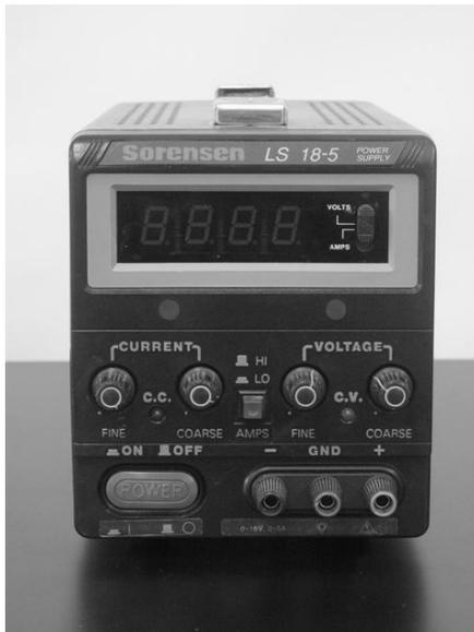
The Sorensen power supply is an all-purpose power supply for the production of constant currents and voltages.
