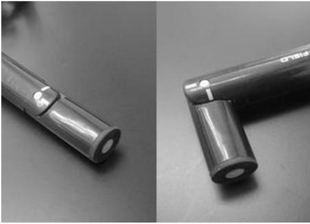
The measurement probes have swiveling tips to allow for more convenient data collection. Note: **these tips are only meant to swivel in one direction. They will break if they are bent in the wrong direction, and they are very fragile, so it does not take much to do this.** Please be very careful as these are costly to replace.
