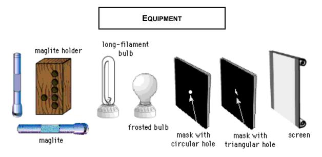
You will have: a maglite holder; two mini maglites; a clear tubular bulb with a straight filament mounted in a socket (representing a long workbench bulb); two cardboard masks, one with a circular hole and one with a triangular hole (representing the holes in the window shade); and a large white cardboard screen (representing the side of the building).
