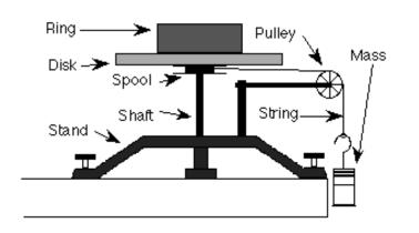
A disk that is mounted on a sturdy stand by a metal shaft. Below the disk on the shaft is a metal spool to wind string around. A metal ring sits on the disk so both ring and disk share the same rotational axis. A length of string is wrapped around the spool and then passes over a pulley lined up with the edge of the spool. A weight is hung from the other end of the string so that the weight can fall past the edge of the table.
