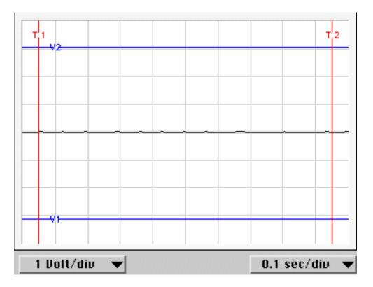
The vertical axis is a measure of the potential difference (voltage) between the two clips. The horizontal axis measures time. You should also notice that the display has a grid on it. The scale of each axis is shown at the bottom of the display. As you might suspect, it is possible to change the grid size of each axis. To change the voltage, click on the "1 Volt/div" and choose from the available choices. Similarly, click on "0.1 sec/div" to change the time magnification.
