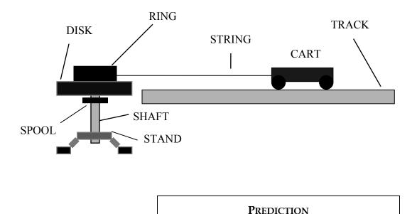
Calculate the angular speed of the disk as a function of the speed of the string and the radius of the ring.
