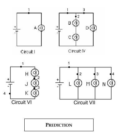
Rank the brightness of the bulbs A, B, C, D, H, J, K, L, M, and N from the brightest to the dimmest (use the symbol '=' for "same brightness as" and the symbol '>' for "brighter than"). Write down your reasoning.
