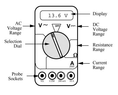
The DMM can measure currents anywhere from 10 amps to a microamp (10<sup>-6</sup> amps). This versatility makes the DMM fragile, since measuring a large current while the DMM is prepared to measure a small one will certainly harm the DMM. For example, measuring a 1 ampere current while the DMM is on the 2 milliamp scale will definitely blow a fuse! If this happens, your instructor can change the fuse. However, if you damage the DMM beyond repair, you will have to finish the lab without the DMM.
