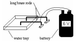
To measure the electric field from the charged electrodes, you will use a probe connected to a digital multimeter set to measure volts (see Figure 2, below). For best results, turn the DMM to measure in the two-volt DC range, as indicated in Figure 2.
