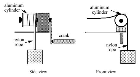
While the cylinder is revolving, the friction between the cylinder and rope is the force holding up the block. An electronic thermometer is embedded into the cylinder. It is read out with a digital multimeter (DMM).
