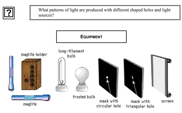
You will have: a maglite holder; two mini maglites; a clear tubular bulb with a straight filament mounted in a socket (representing a long workbench bulb); two cardboard masks, one with a circular hole and one with a triangular hole (representing the holes in the window shade); and a large white cardboard screen (representing the side of the building).
