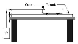
You will be able to vary the mass of Object A (the "mass hanger") and the Cart. They are connected together using a light string. Object A falls through a distance which is significantly shorter than the length of track. You will have a meter stick, a stopwatch, a mass hanger, a mass set, cart masses, a pulley, a pulley clamp, one piece of string and the video analysis equipment. In this experiment we ignore the friction between the cart and the track.
