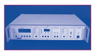
The ITC503 is an intelligent temperature controller, with general applications in the temperature range 0.3 to 1500 K. It will accept a wide range of standard sensors as well as many custom calibration ranges. Standard ranges are held within the non-volatile memory of the individual instrument while custom ranges are linearised and loaded easily and accurately via Object Bench Software.
